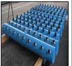
Job - Description: Boiler main drums, LP drums, Headers, Boiler Ring Headers.
